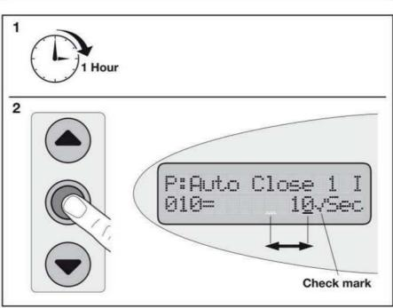
Press the Up and Down arrows to change the parameter value displayed to the value you have selected from the parameter list. The Up arrow increases the parameter value, and the Down arrow decreases the parameter value.
